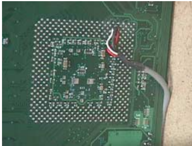
Figure 7-15. Back side of motherboard with PGA370 connections
